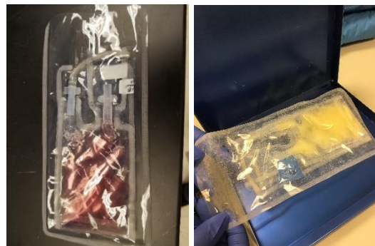
Fig. 4 (left) KryoSure® Bag assembly contained in overwrap (right) KryoSure® Bag in cassette after freezing
